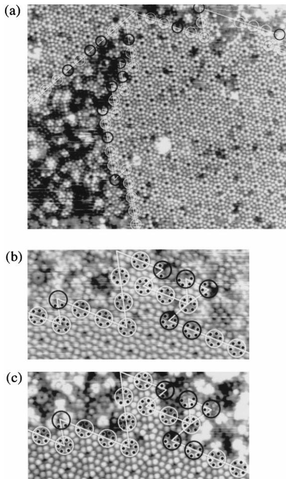
Fig. 11. (a) STM image of a quenched Si(111) surface ( $V_s = -2.0$  V,  $I_t = 0.3$  nA). Characteristic structure of the boundary with (b) positive ( $V_s = 2.0$  V,  $I_t = 0.3$  nA) and (c) negative ( $V_s = -0.5$  V,  $I_t = 0.3$  nA) bias voltages. Corner holes at the boundary with complete and incomplete structures are indicated by white and black circles respectively.
