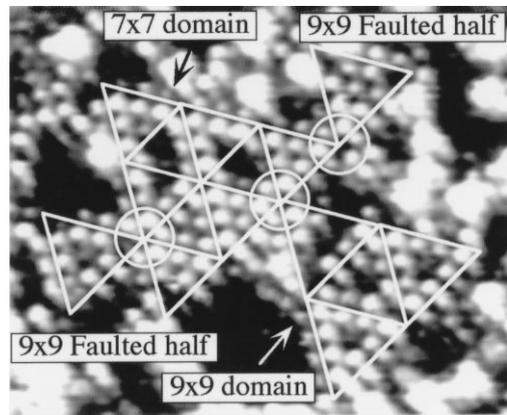
Fig. 7. STM image of a quenched Si(111) surface ( $V_s = -0.5$  V,  $I_t = 0.3$  nA). Three  $9 \times 9$  domains exist sharing corner holes with a  $7 \times 7$  triangular domain.
