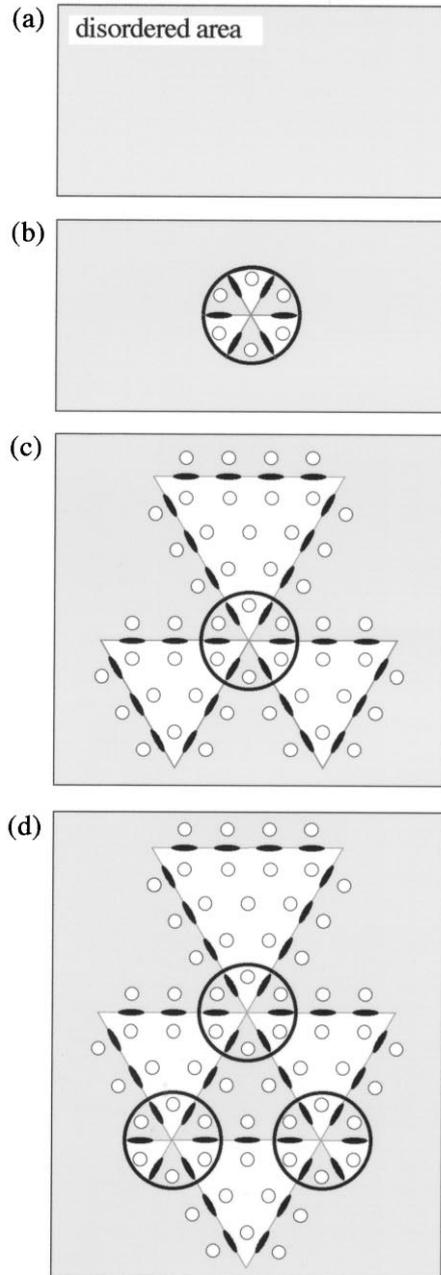
Fig. 8. Schematic diagram of the formation process of the DAS structure: (a) high-temperature disordered area, (b) nucleation of a corner hole, (c) growth of half-unit cells of DAS structures including an SF from the corner hole and (d) complete formation of the DAS structure.
