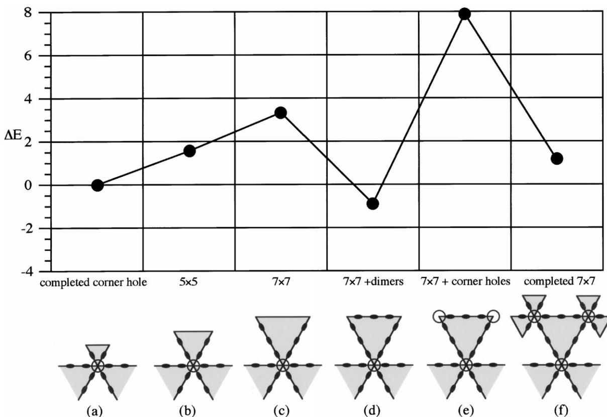
Fig. 10. Schematic of the formation of  $7 \times 7$  SF half-cell. The change in the relative structural energy is also shown.
