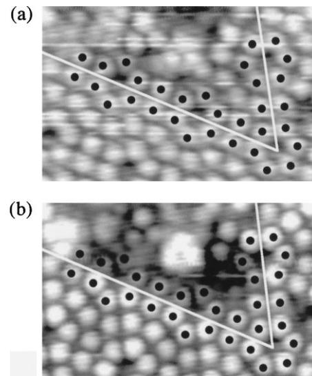
Fig. 3. Magnified images of a boundary between  $7 \times 7$  and disordered areas taken at positive and negative bias voltages are shown in (a)  $V_s = 2.0$  V,  $I_t = 0.3$  nA and (b)  $V_s = -0.5$  V,  $I_t = 0.3$  nA respectively. Adatoms at the boundary are indicated by dots.
