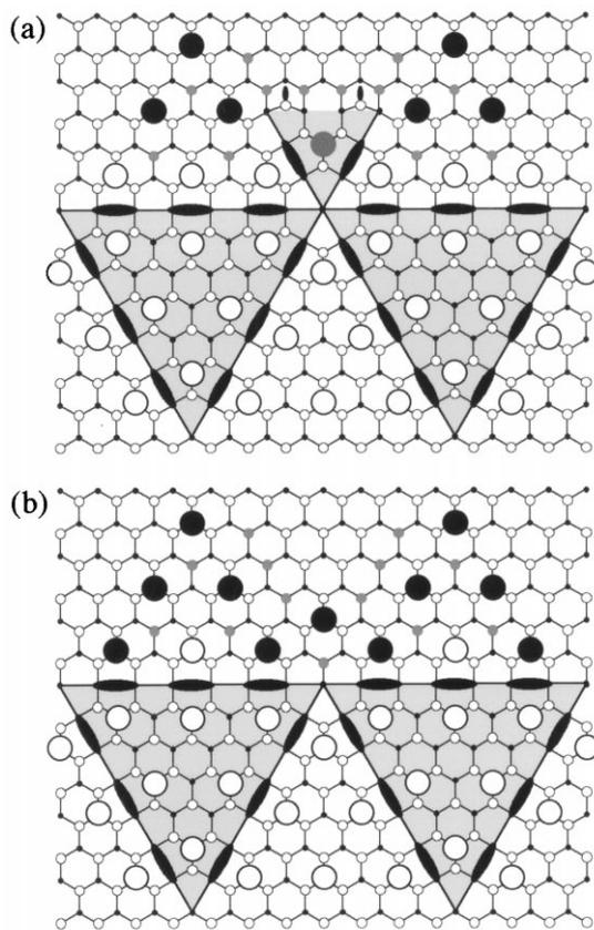
Fig. 2. Schematics of the domain boundary between the  $7 \times 7$  and disordered areas, in which (a) an SF is formed and (b) not formed. Bright and dark adatoms and under-layer dimers are indicated by open and filled circles, and closed ellipses respectively.
