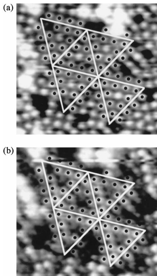
Fig. 5. STM image of a  $9 \times 9$  domain structure on a quenched surface. (a)  $V_s = 2.0$  V,  $I_t = 0.3$  nA and (b)  $V_s = -0.5$  V,  $I_t = 0.3$  nA. Adatoms at the boundary are indicated by dots.
