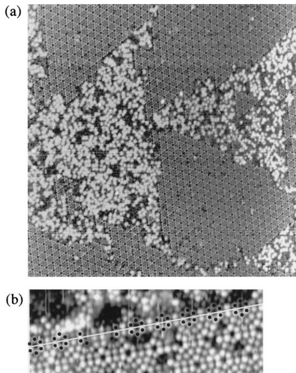
Fig. 1. (a) STM image of a quenched Si(111) surface ( $V_s = -2.0$  V,  $I_t = 0.3$  nA), and (b) a magnification of a boundary between the  $7 \times 7$  and disordered areas.
