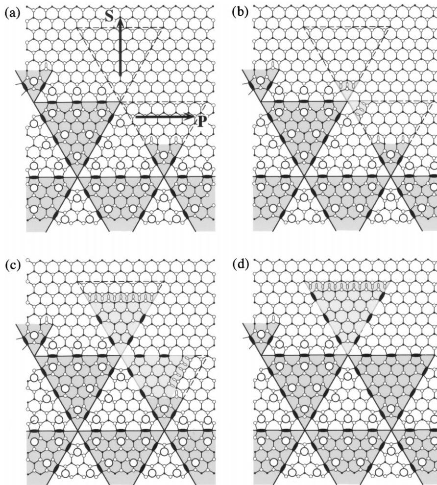
Fig. 13. A schematic of the recombination process of each Si-bond in the formation of an SF unit by the P- and S-processes shown in Fig. 12b.
