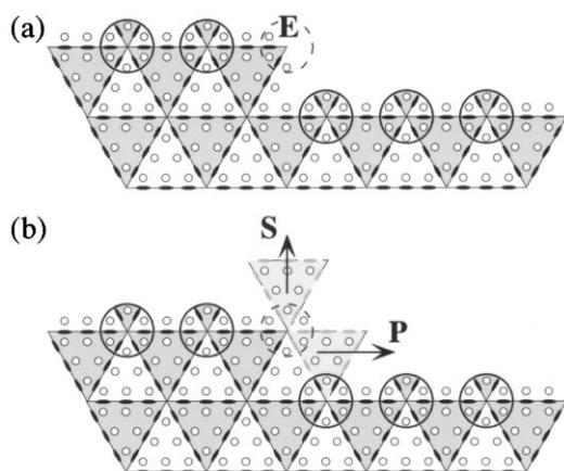
Fig. 12. (a) Schematic of the boundary structure in Fig. 11. E indicates an edge of the SF unit in the domain. (b) Two possible growth processes for an SF unit from the edge E in (a).
